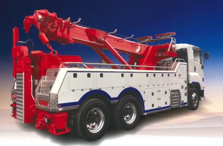
World's first 360° rotational winch boom. Any work is possible with the 3-stage long boom and double wrench. The under lift tows from light passenger vehicles to small-sized trucks.
